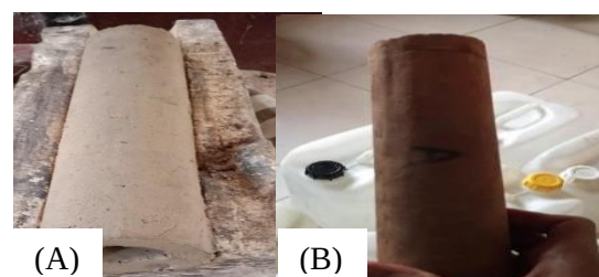
Figure 4. Ceramic Membrane (A) with Rice Husk Additives, (B) without Rice Husk Additive
