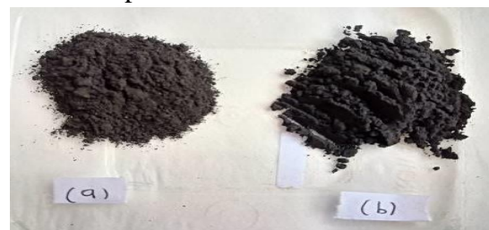
Figure 1. (a) Carbon before activation, (b) Activated carbon
