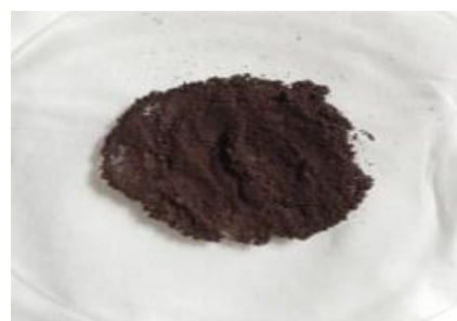
Figure 3. Activated carbon after being layered with MnO 2 (AC/MnO 2 )
