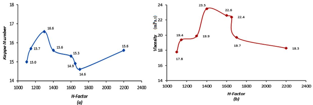
**Figure 3.** (a) Relationship between H-Factor and Kappa Number, (b) Relationship between H-Factor and Viscosity at a Production rate of 1300 ADT/d
