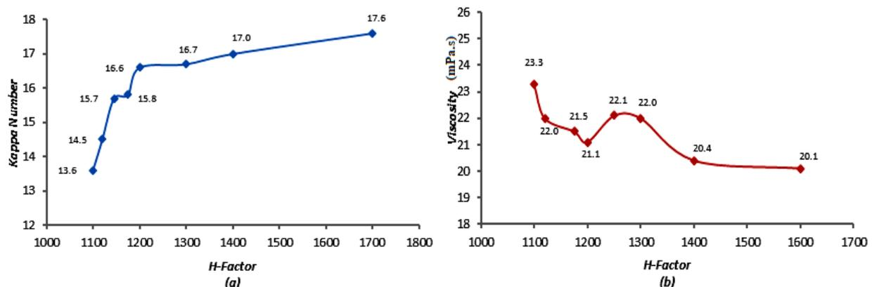
**Figure 5.** (a) Relationship of H-Factor and Kappa Number, (b) Relationship of H-Factor and Viscosity at a Production rate of 1500 ADT/d
