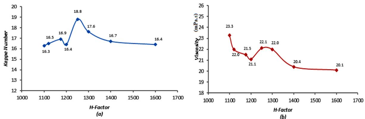
**Figure 4.** (a) Relationship of H-Factor and Kappa Number, (b) Relationship of H-Factor and Viscosity at a Production rate of 1400 ADT/d
