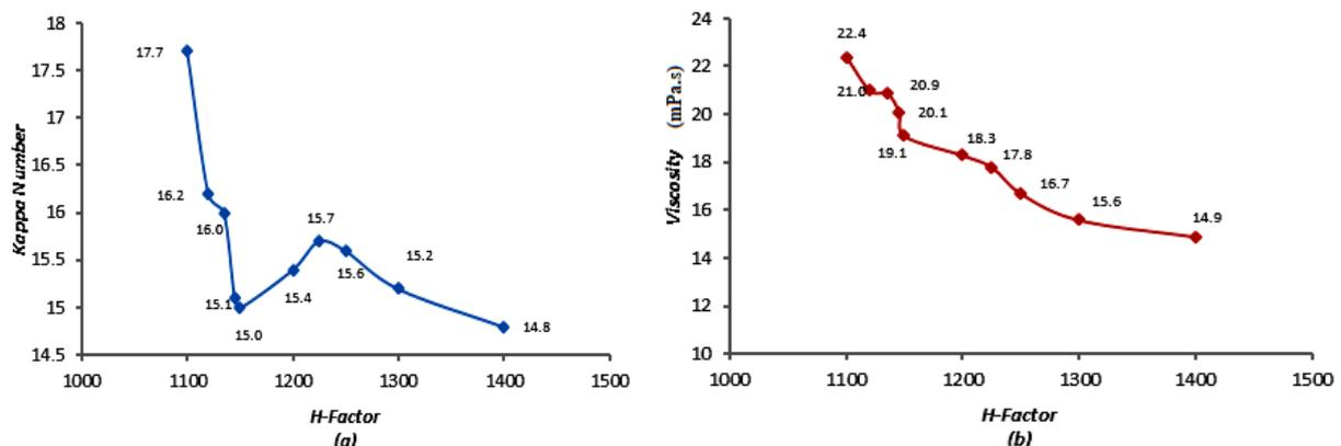
**Figure 6.** (a) Relationship of H-Factor and Kappa Number, (b) Relationship of H-Factor and Viscosity at a Production rate of 1600 ADT/d
