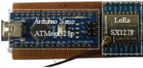
Gambar 5. Purwarupa Wearable Device Penerima Data
